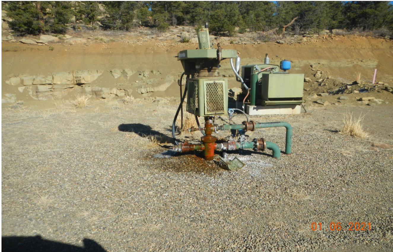
Photo 4. Water is leaking from the wellhead.
