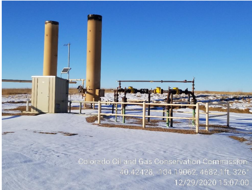
Photo 3 – Gas Meter, ECDs
