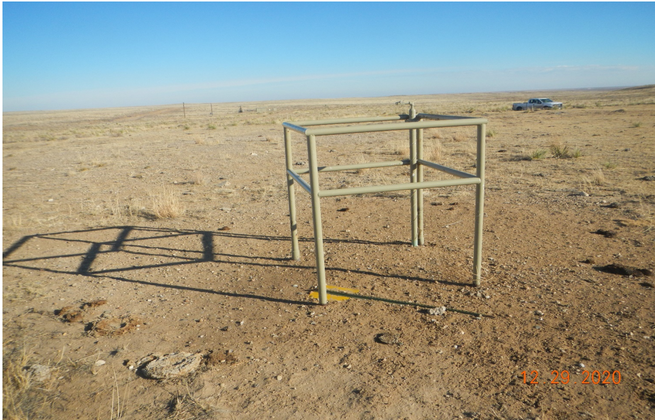
Photo 5. There is another pipe riser that remains at the center of the location. All equipment should have been removed within 3 months of abandonment of the well.
