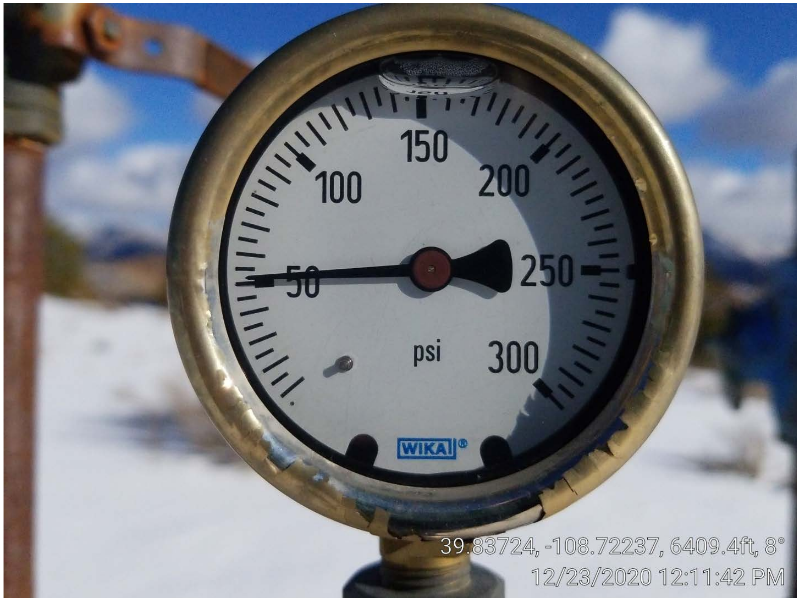
Photo 3. Casing gage.
