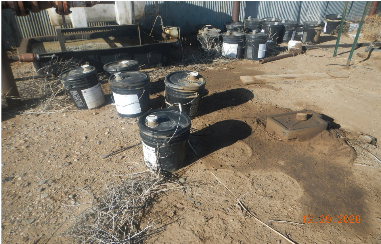
Photo 5. There is oil stained soil from spills that have occurred. There are several containers that are not labeled and appear to contain oil.
