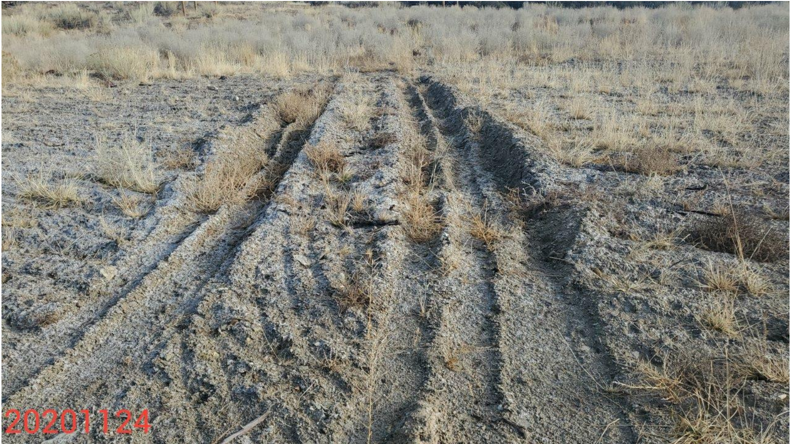
Photo 10: Photo taken from the Location, facing east. Photo shows vehicle travel on the location has resulted in deep ruts throughout the reclamation area; Additional reclamation work will be required in these areas to repair rutting, address potential compaction and revegetation concerns resulting from vehicle use.
