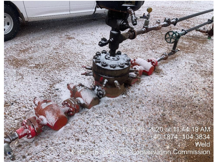
Photo #8 Surface Casing has no Bradenhead provisions (Not Plumbed to Surface)
