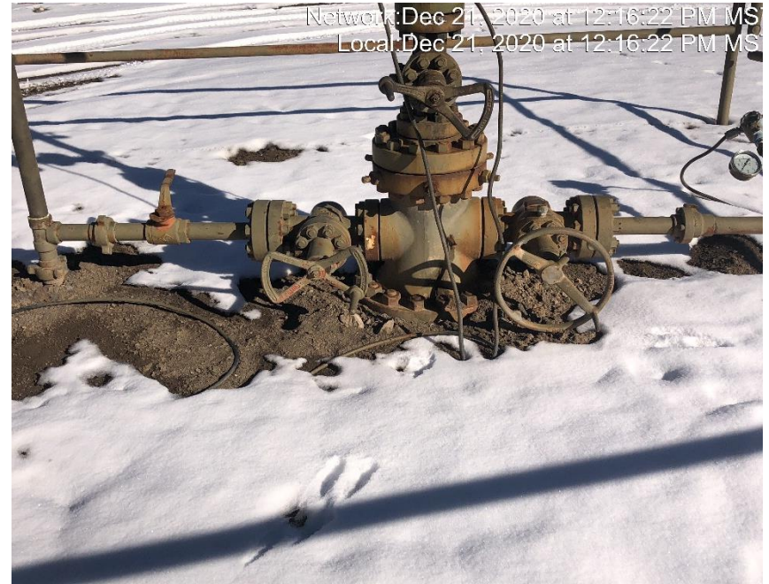
Photo #2507 Braden head valves are not accessible.
