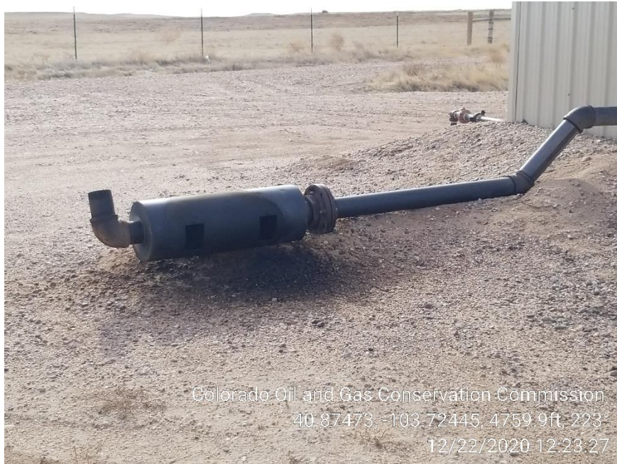
Photo 5 – Stained Soil at Exhaust
