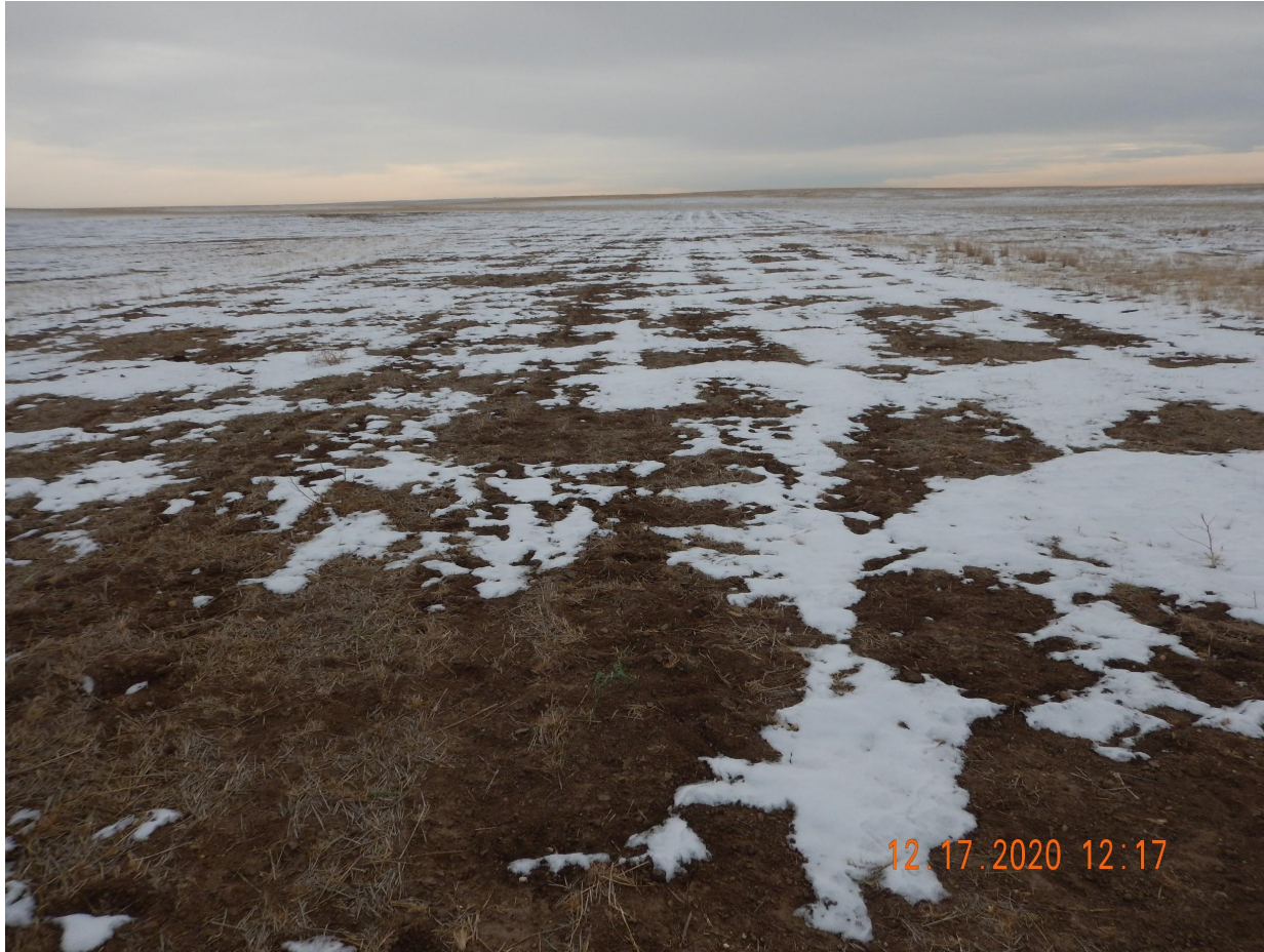
Photo 1. Photo taken from the entrance of location, facing South. Photo illustrates the location does not appear to meet Rule 1004 vegetative standards. The vegetation-like material in the photo is not actually vegetative growth but straw mulch used during final reclamation activities. There was sparse desirable vegetation observed throughout the location, which is not reflective of reference area vegetation.
