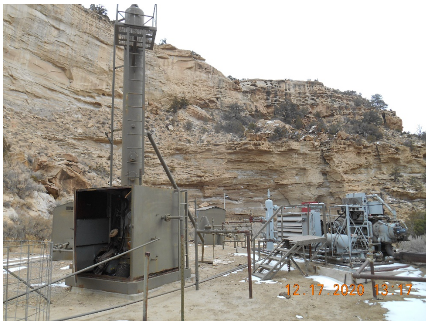
Dehydrator and compressor
