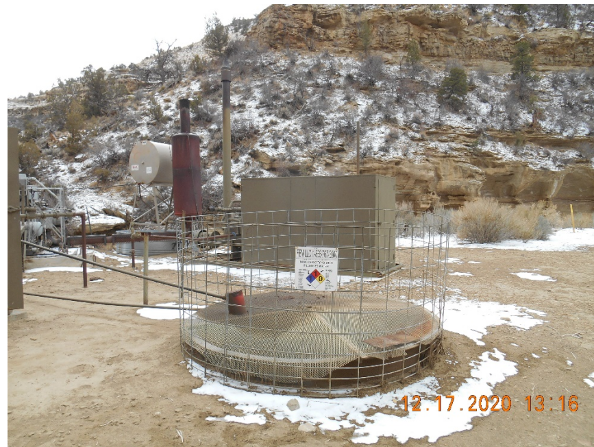
Separator and blowdown tank
