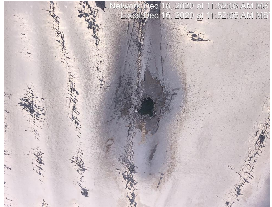
Photo #2480 Multiple holes in tank containment liner.
