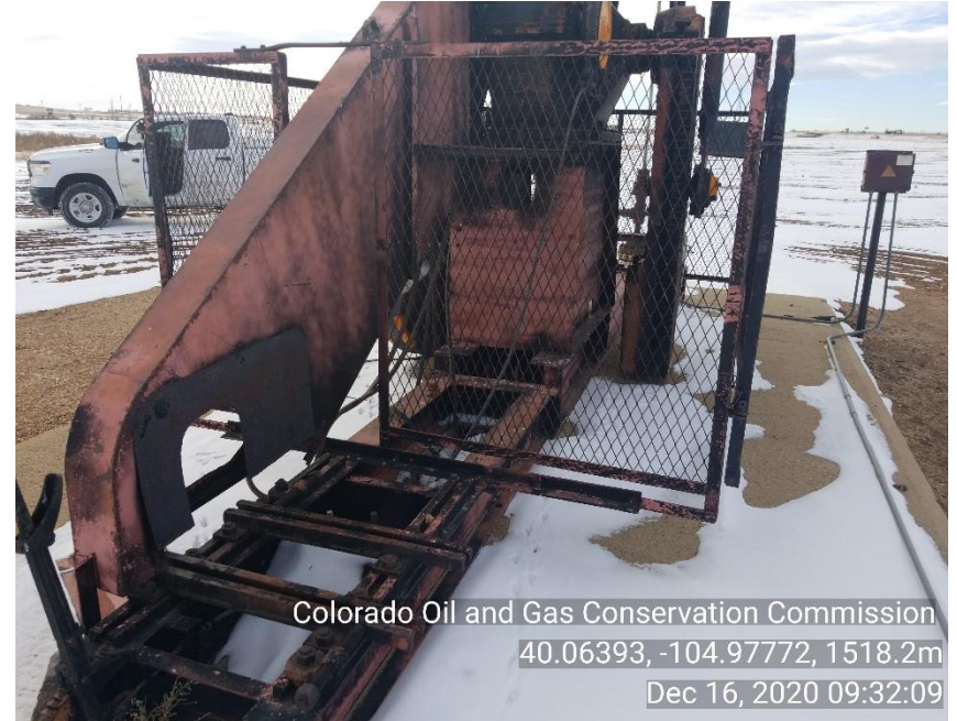
Photo 2 no motor on PU, UNUSED EQUIPMENT
