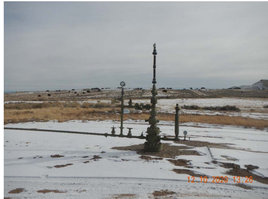
Photo 2. No bradenhead access apparent.
