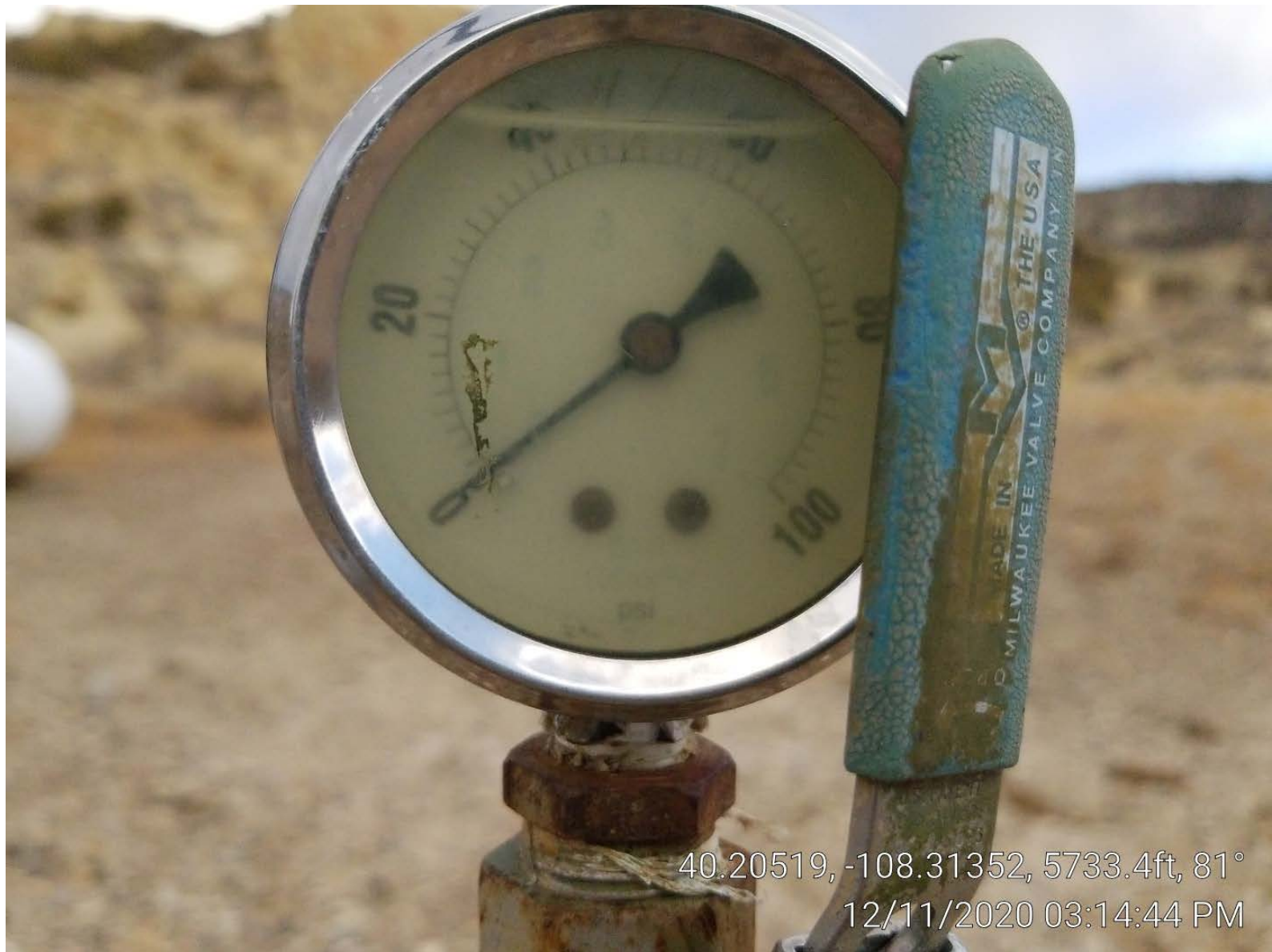
Photo 17. Casing gage.
