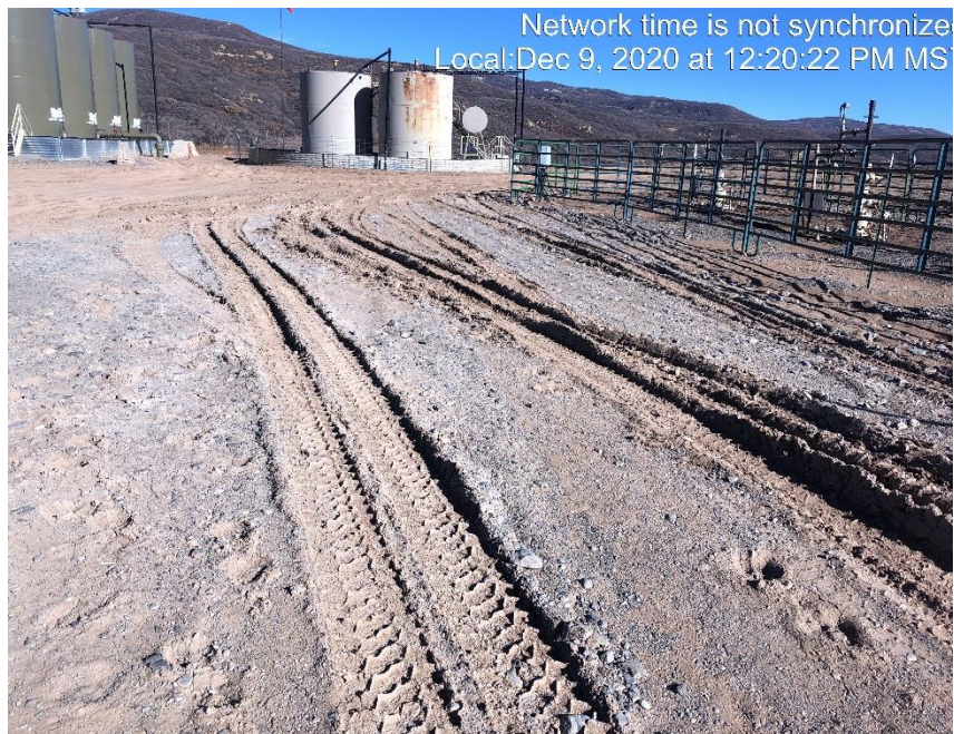
Photo #2434 Sediment is being transported off of location
