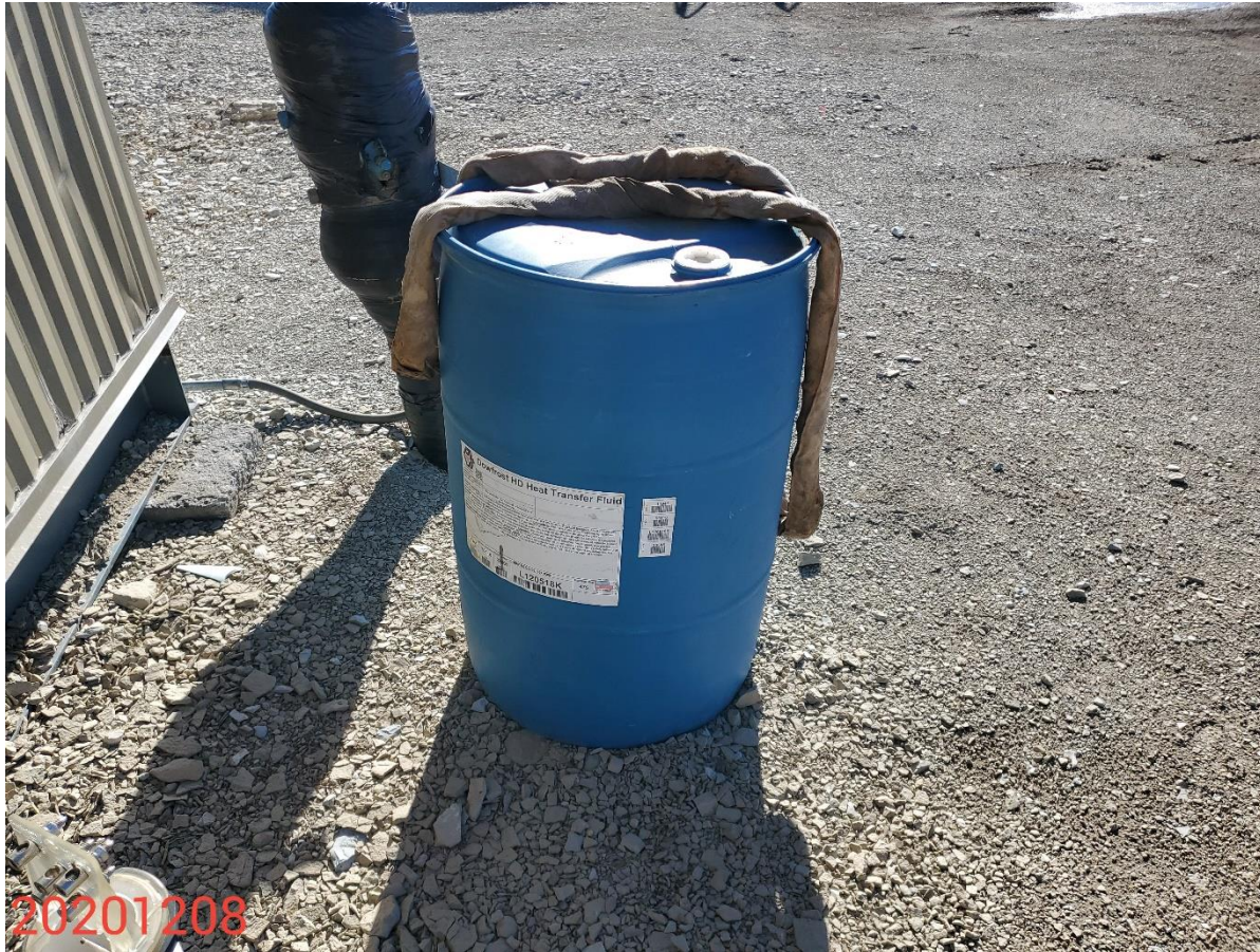
Photo 6: Shows barrel containing “heat transfer fluid” stored on the location. This is not proper materials management; Place barrel into secondary containment, or remove and properly stored.
