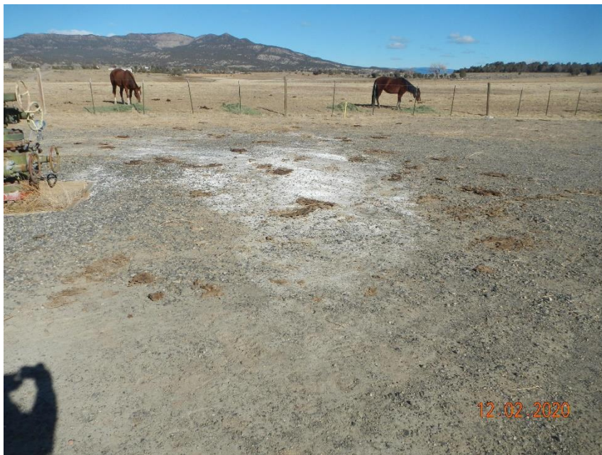
Mineral crust in flat area indicative of produced water release
