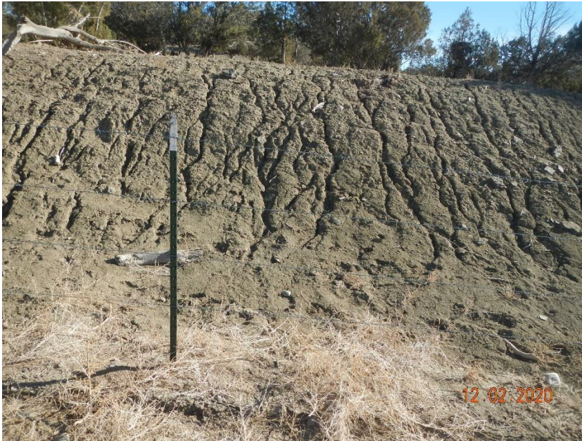
Looking east, rill erosion on bermed slope on east side of location
