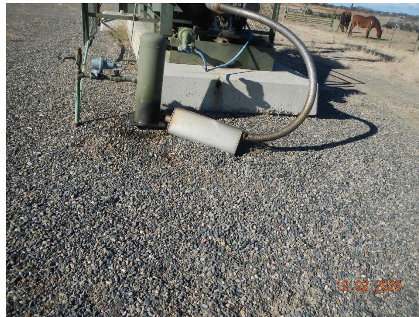
Exhaust leak
