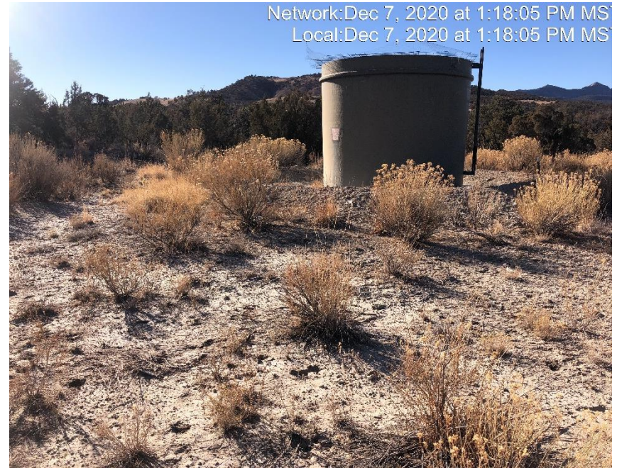
Photo #2418 Vegetation growing on secondary containment.
