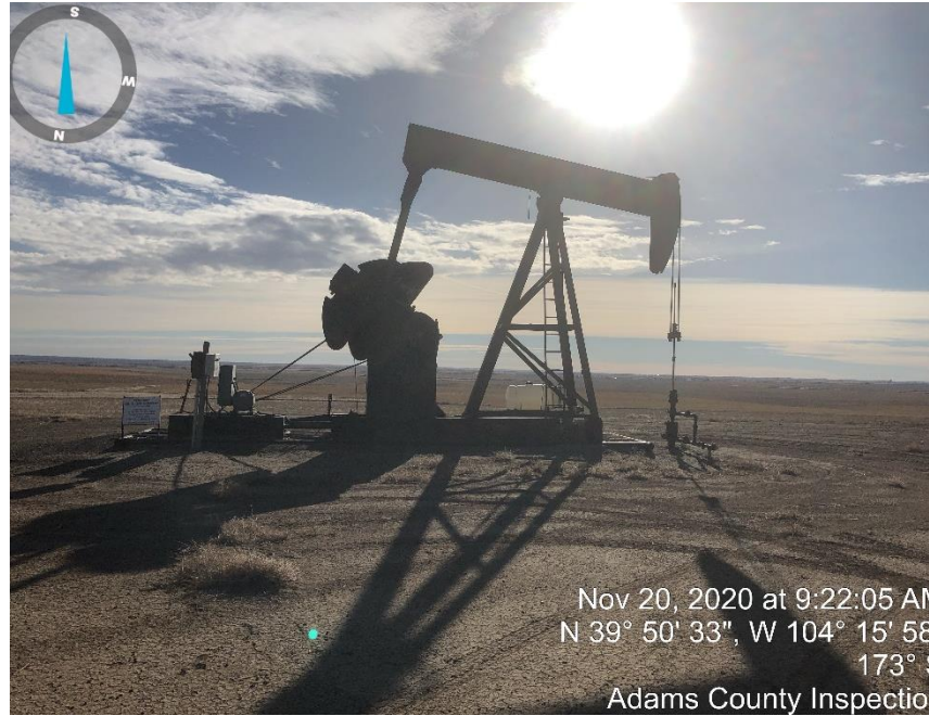
Photo #1 Pump Jack.
