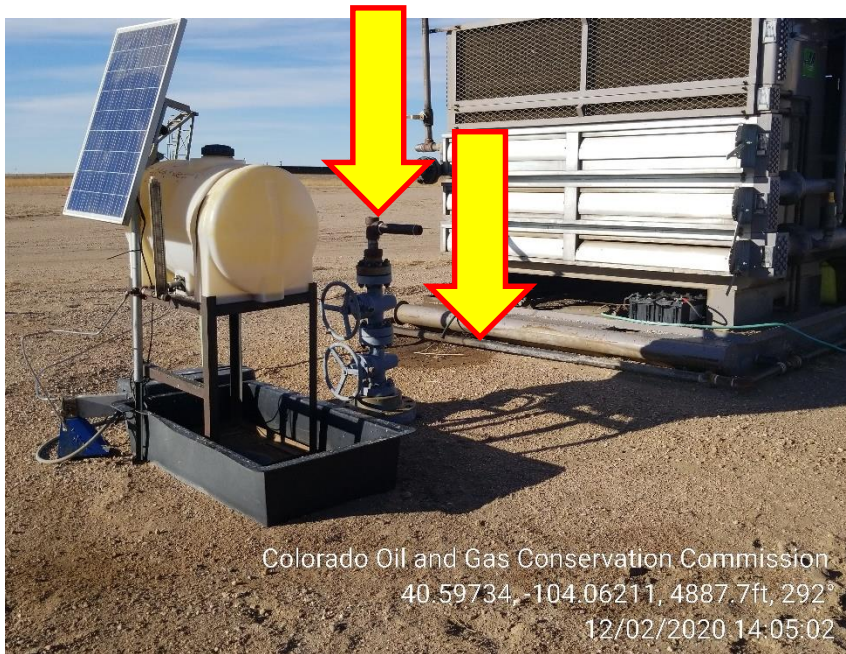
Photo 15 – Stained Soil at Compressor and Unused Parts
