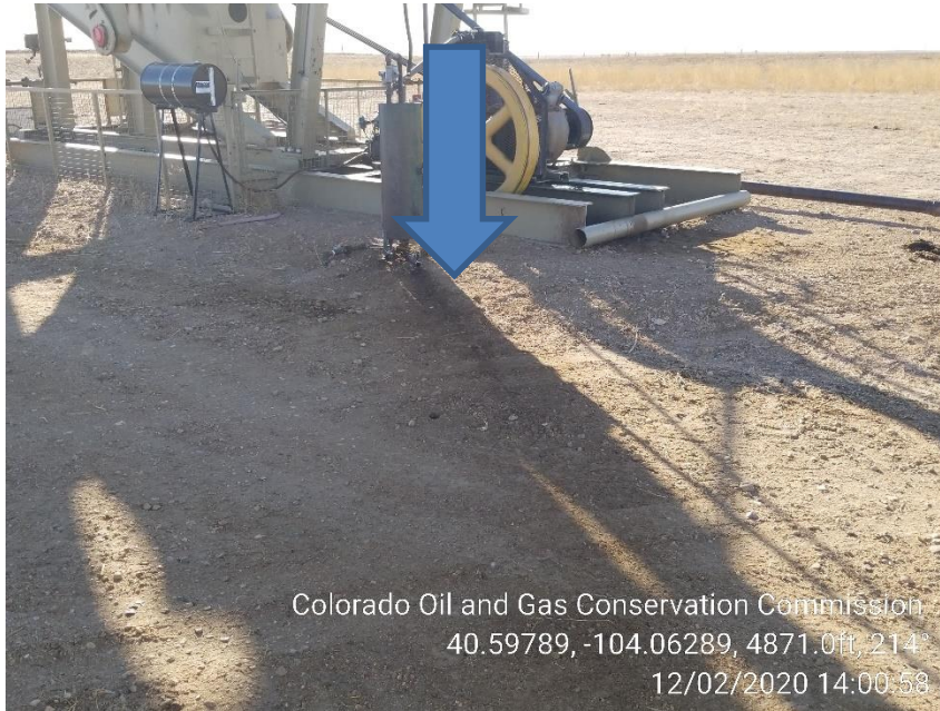
Photo 9 – Stained Soil at 2-1H Supply Pot
