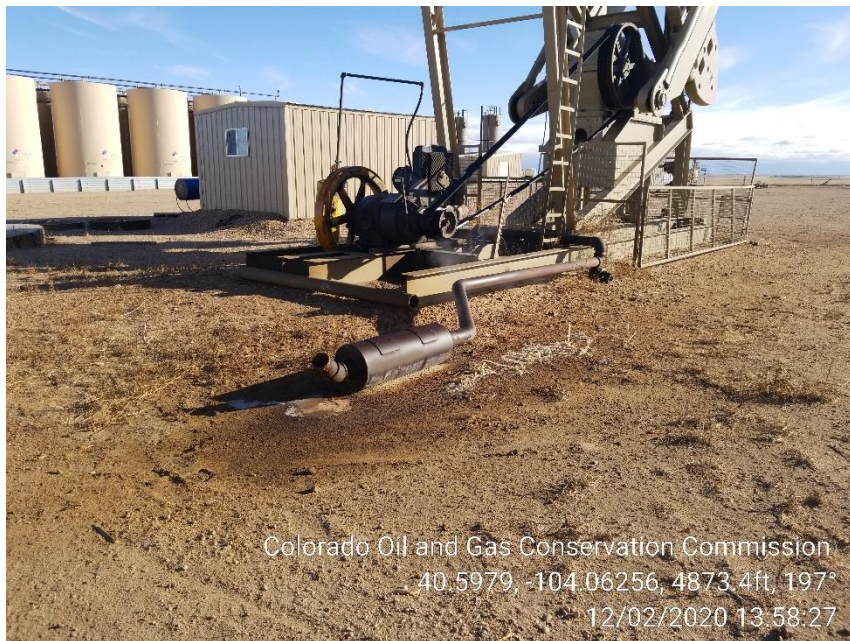
Photo 5 – Stained Soil at 2-3H Exhaust
