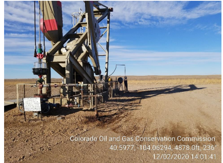
Photo 10 – Stained Soil at 2-1H Wellhead
