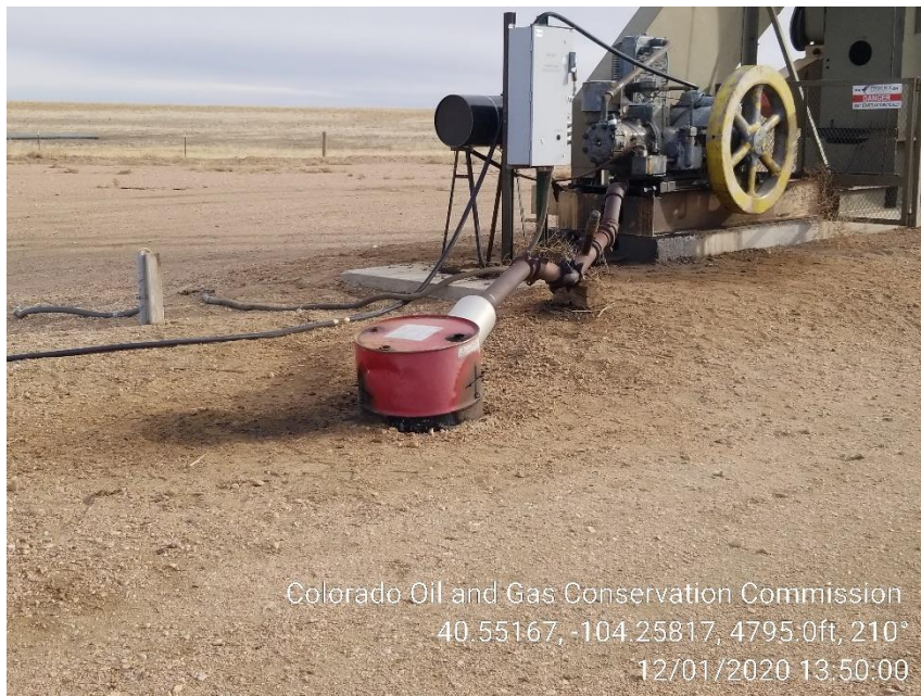
Photo 5 – Stained Soil at Exhaust
