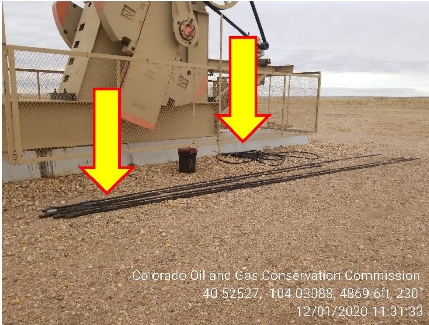
Photo 7 – Unused Rods and Belts at Pumping Unit
