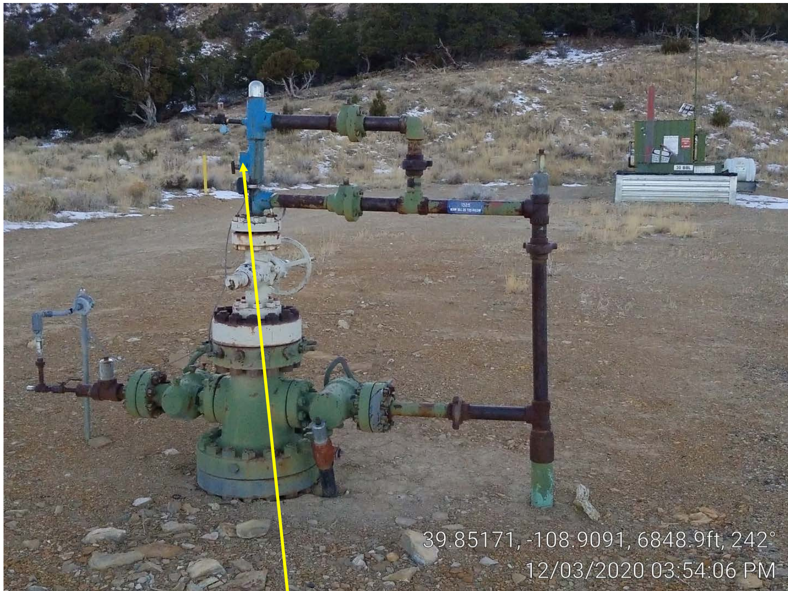
Photo 2. Location with gas leak.
