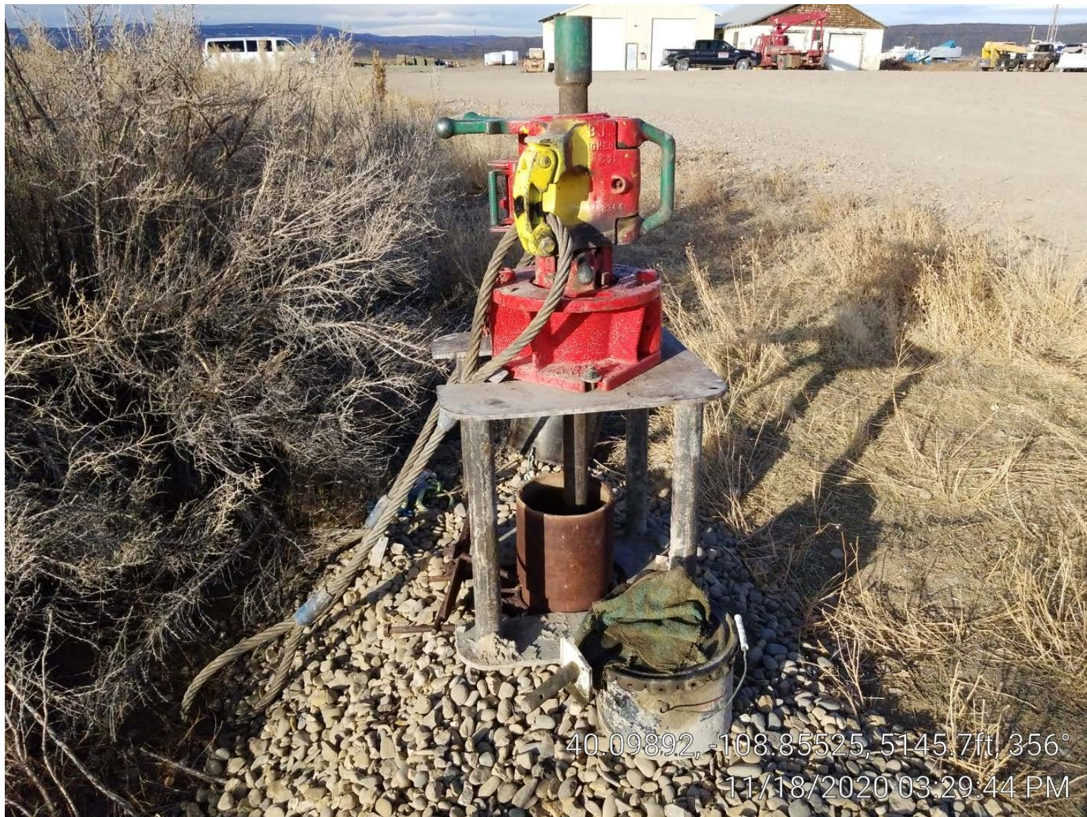
Photo 2. Temporary tubing in place used to pump cement downhole.
