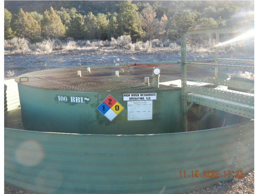
Open topped produced water vessel.
