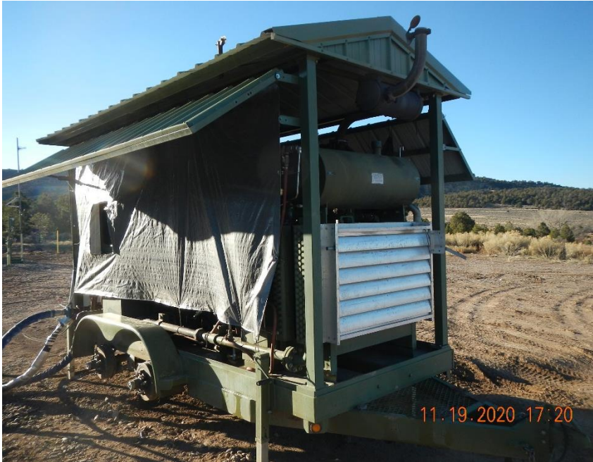
Trailer mounted compressor.
