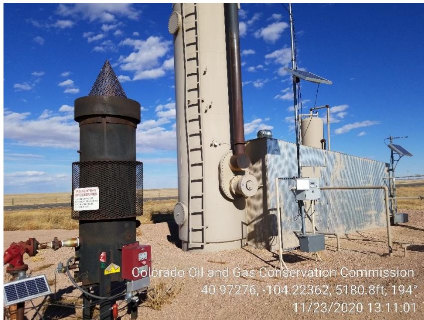
Photo 3 – Heater Treater, ECD
