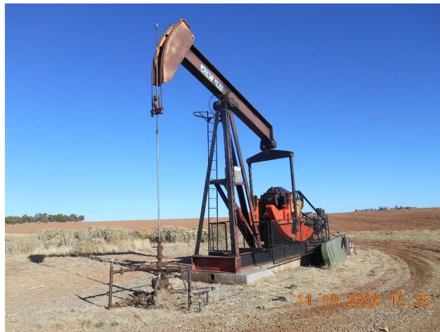
Wellhead with Pump Jack
