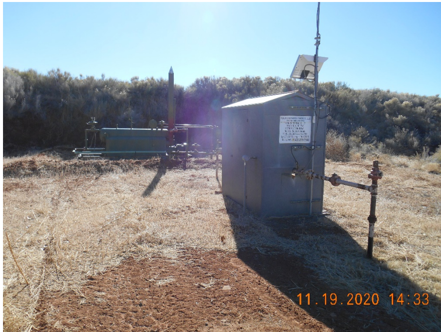
Meter housing with sign and Separator with earth berms
