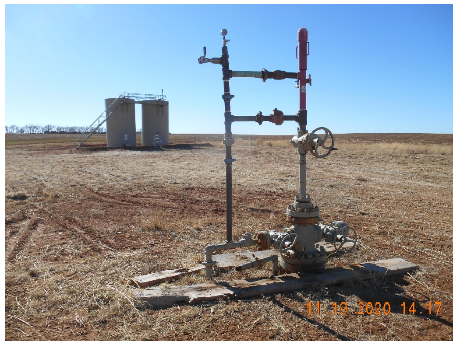
Wellhead with plunger lift.
