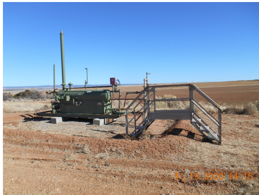
Separator with earth berms.
