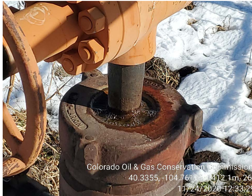
Wellhead packing leak
