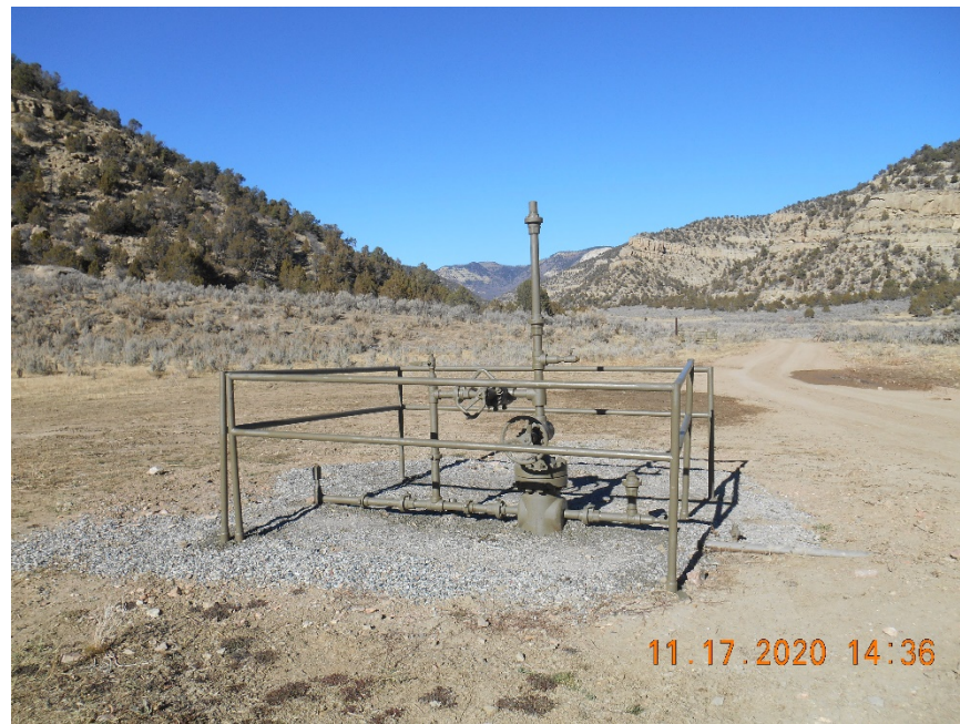
Wellhead with fence
