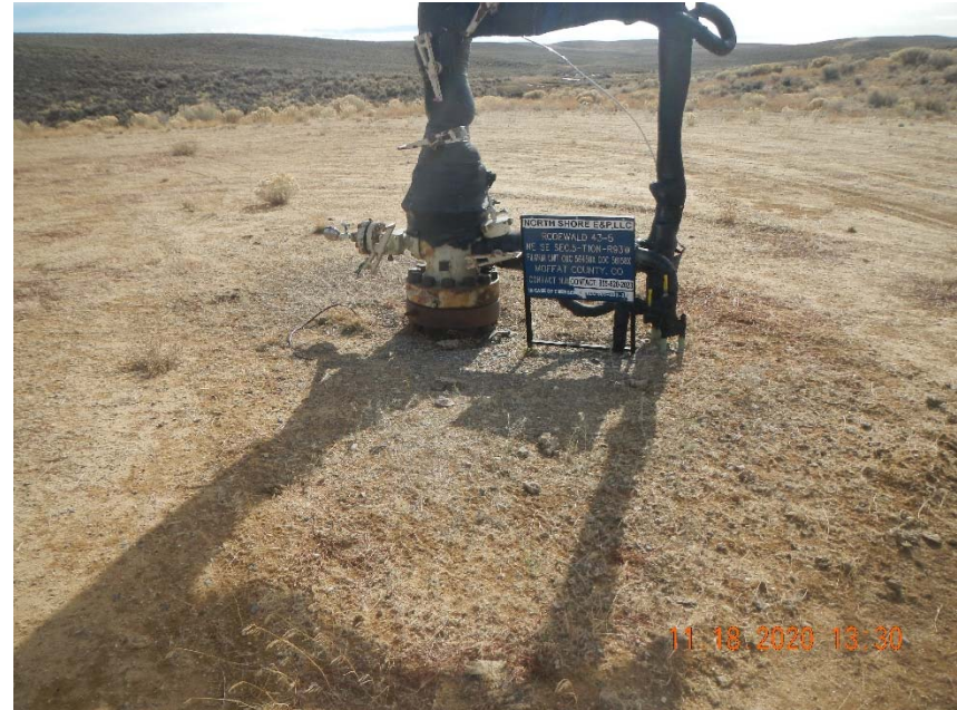
Photo 2. No bradenhead access apparent.
