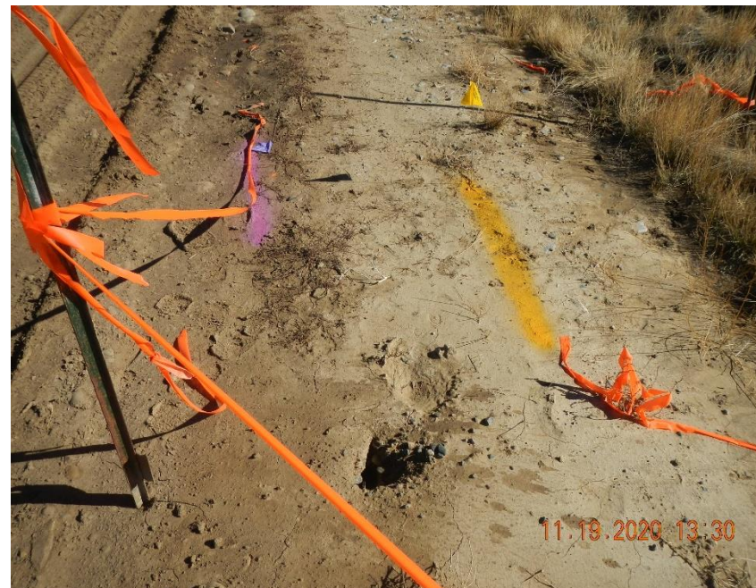
An approximately 6" diameter hole was observed within the area marked.
