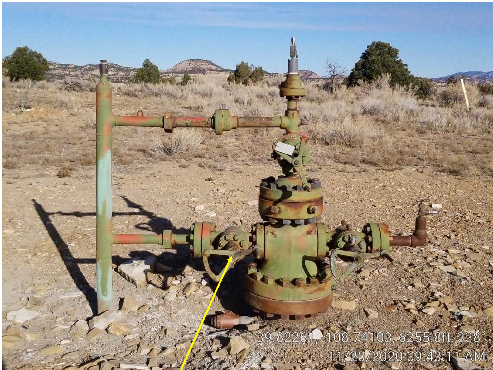
Photo 2. Well with gas leak.
