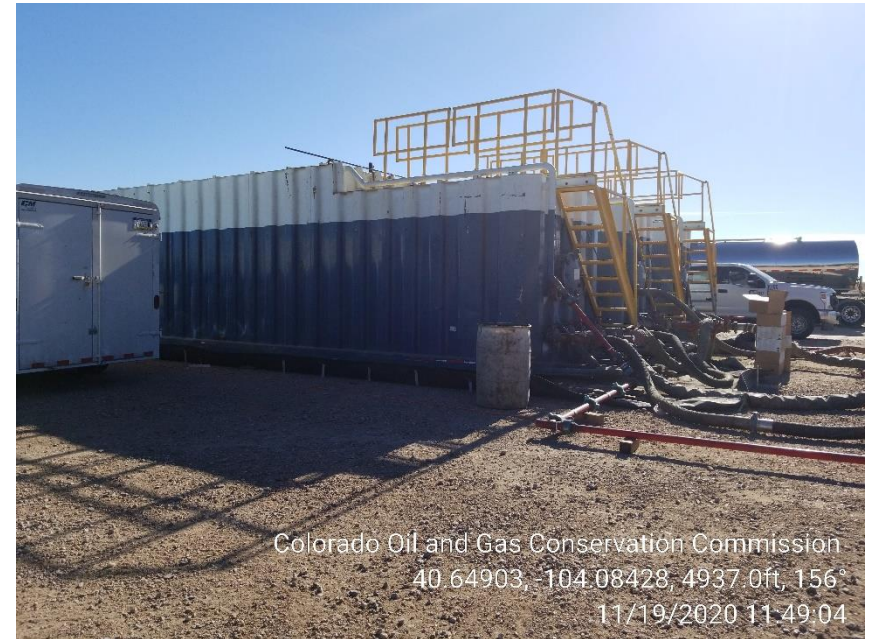
Photo 2 – Fresh Water and Flowback Tanks not grounded
