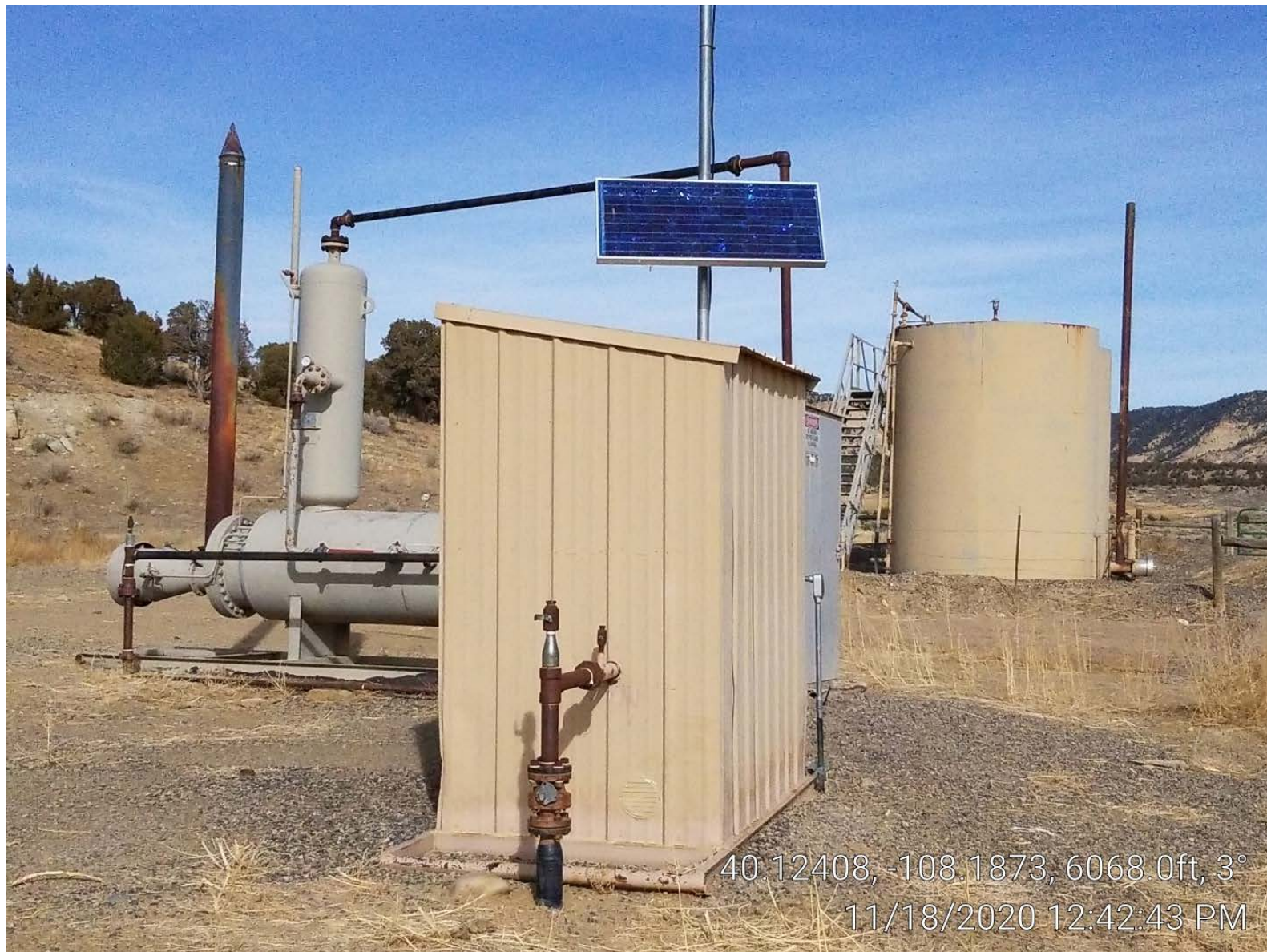
Photo 3. Meter building, separator, tanks.
