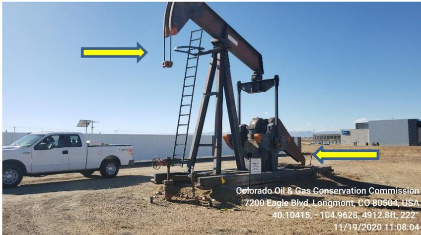
**Photo 3 pump jack not connected to well and no power**
