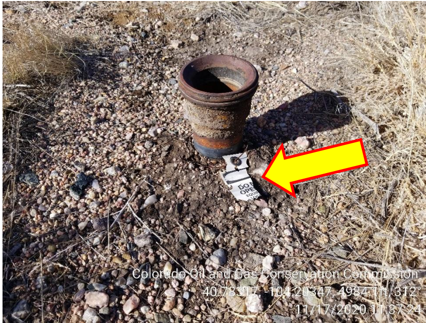
Photo 5 – Unmarked Risers
