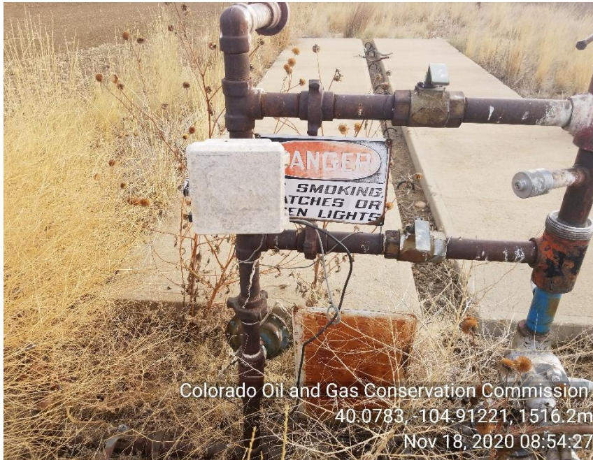
Photo 3 all flow line valves off well head are closed.
