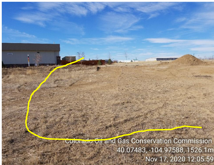
Photo 1 Disturbed area from spill remediation. No BMP's in place
