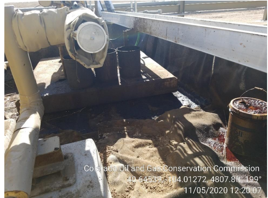
Photo 10 – Oily Waste at Re-Cycle Pump
