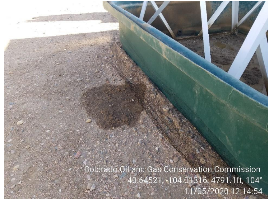
Photo 8 – Stained Soil at Compressor Day Tank
