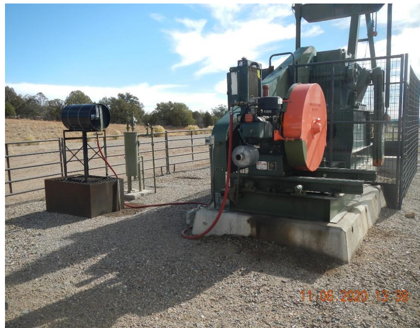
Stained concrete pad and gravel beneath prime mover at the AA #4 pump jack.
