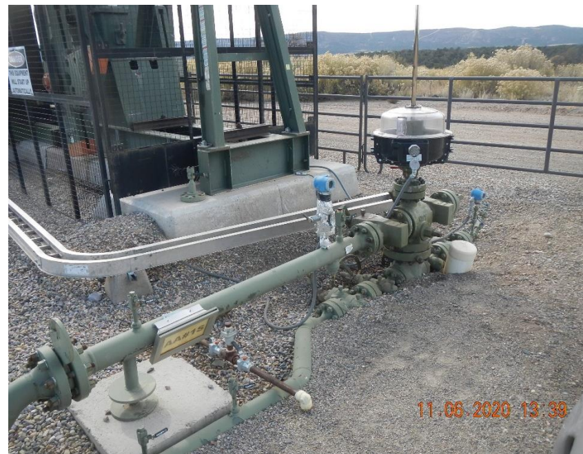
"Trapper" stuffing box containment device at the AA #1S.
