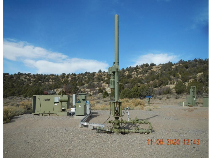
Beuten B #1 well head and artificial lift equipment.
