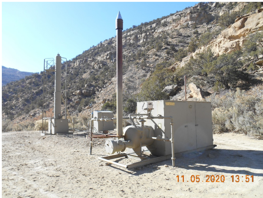
Separator, Dehydrator and Meter housing
