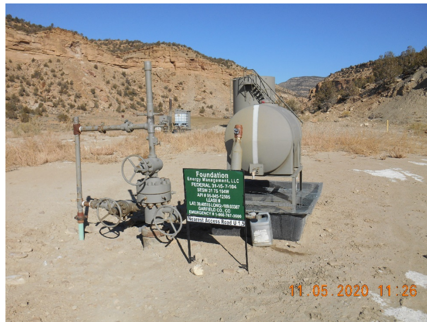
Wellhead with chemical injection tank
