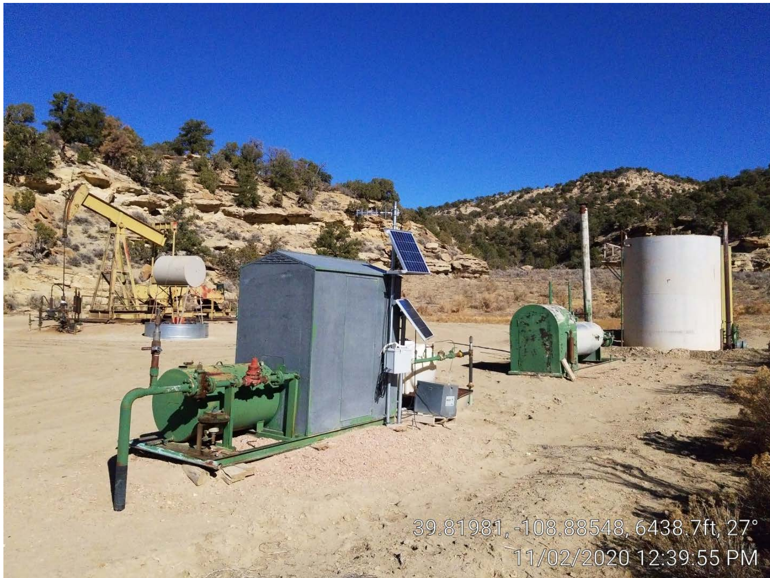
Photo 3. Meter building separator, pump jack, tanks.
