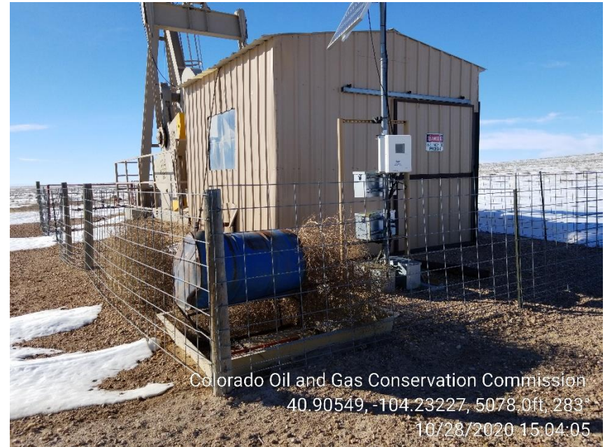
Photo 2 – Unused Chemical Tank and Containment
