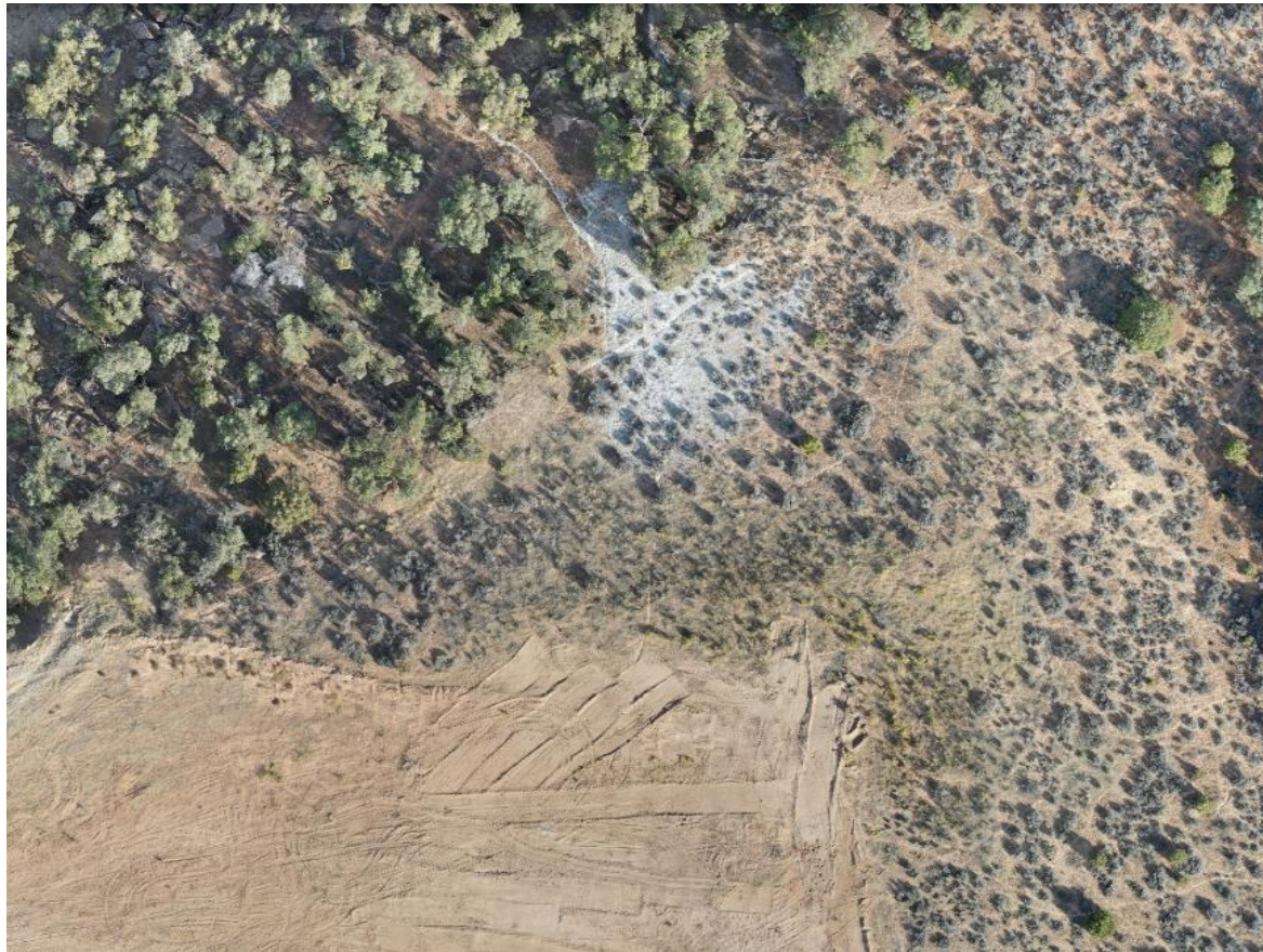
Photo 16: Aerial image of the Location collected date-of-inspection via a sUAS. Photo shows spill area/impacted soils on the north end of the location. Area measuring ~0.11 acres in size.
