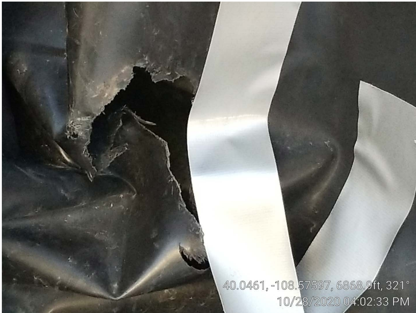
Photo 5. Secondary containment liner hole.
